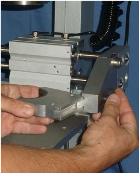
**Figure 17: Setup – Attaching clamps**
