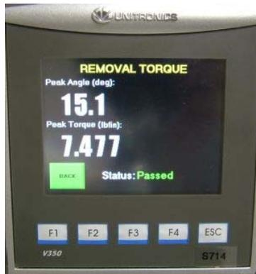
Figure 31: Test – Numeric Display
