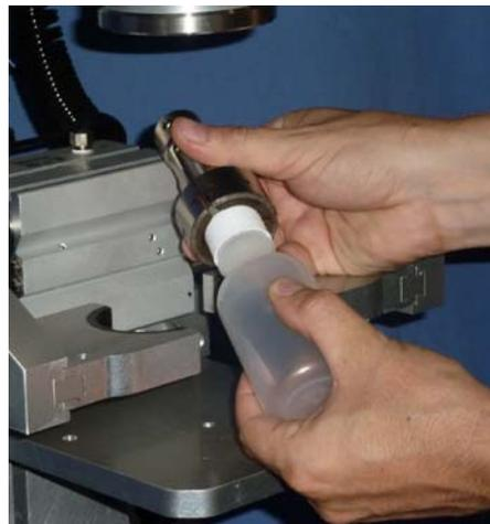
Figure 13: Setup – Finding the collet
