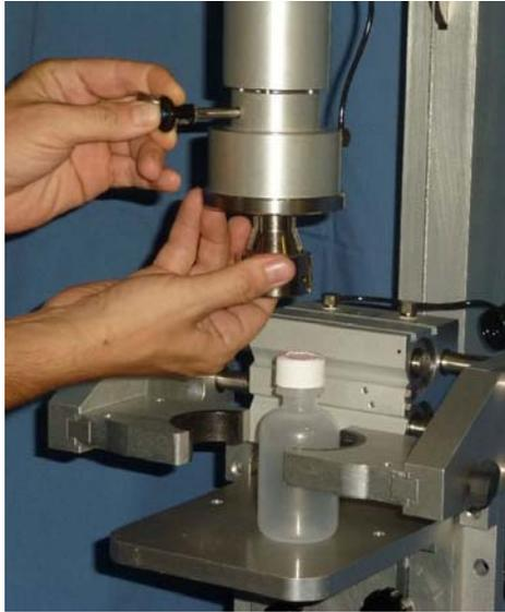
**Figure 19: Setup – Securing the collet**
