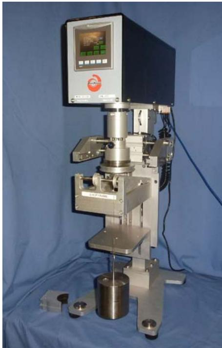
Figure 9: Calibration – Mechanical Setup for CCW calibration
