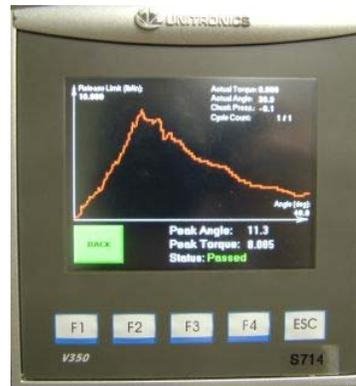
Figure 32: Test – Graphical Display
