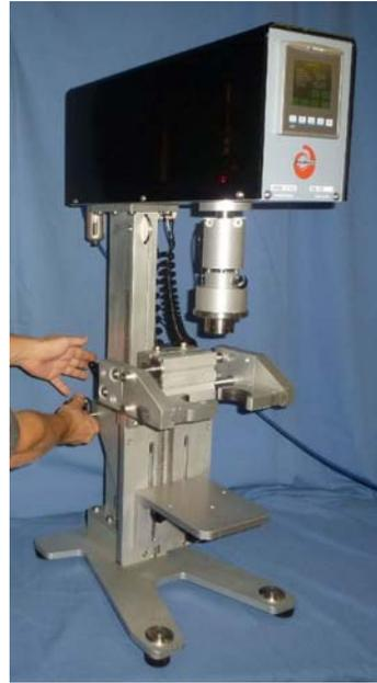
**Figure 16: Setup – Lowering platform assembly**
