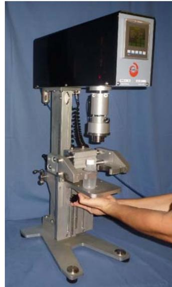
**Figure 18: Setup – Platform height adjustment**
