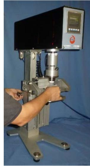
**Figure 20: Setup – Adjusting the platform assembly height**
