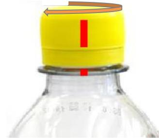
Figure 3. Application Angle Suggests Torque is Close to Target
