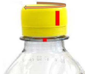
Figure 4. Angle Suggests Torque is too Low
