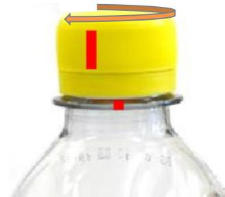
Figure 2. Application Angle Suggests Torque is too High
