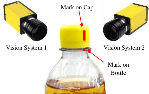
Figure 1. Example Setup: Visual Application Angle Measurement
