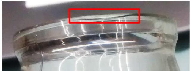
Figure 7. Cracking at the External Edge
