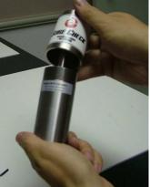
Unscrew the upper part to recover the torque adjustment window.
