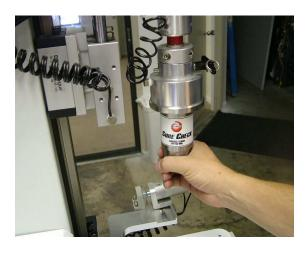
Check calibration of reference ST-LAB with the dead weight method, then insert the SureCheck in the chuck.
