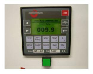
Unless the customer specified otherwise, the SureCheck is calibrated to produce 10lbfin breakaway torque.
