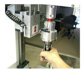
Assemble chuck adapter and SureCheck, then slide it in the chuck, secure it with the quick release pin and check break torque in release mode. If peak is within +/- 0.1 lbfin of the required break torque, take SureCheck out of the chuck, if adjustment is required, repeat previous step.
