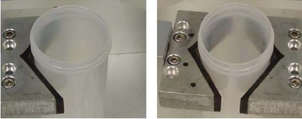
Distortion caused by excessive bottle clamping pressure in an automatic clamping system
