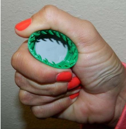
In order to overcome the variation introduced by manual gripping, custom molded, 3d printed or machined “serrated” chucks can be used for securing the caps during the torque test.
