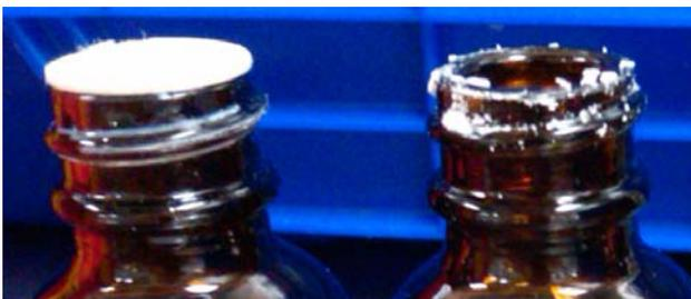
Due to the thread locking properties of such product residue, the release torque readouts can be considerably higher and the product appearance/quality is also adversely affected.
