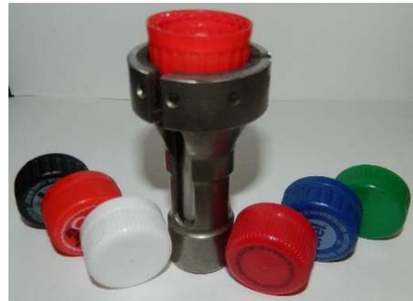
For example, one air actuated chuck size works well for multiple serration types for the same cap diameter and by optimizing the gripping pressure, the removal torque results are comparable to those measured with serrated chucks.
