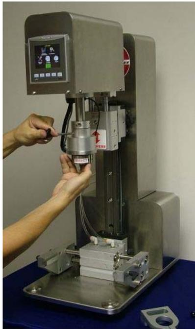
**Figure 19: Setup – Securing the collet**
