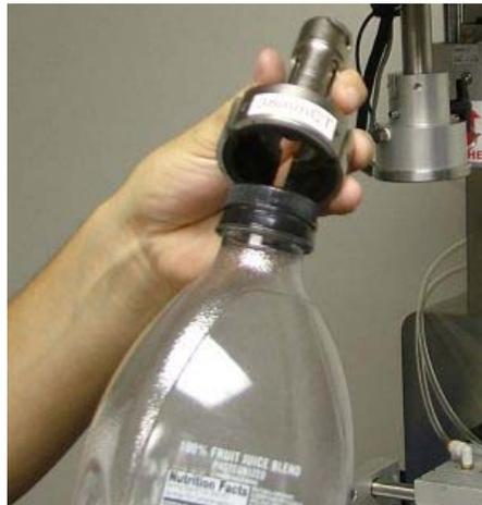
**Figure 13: Setup – Finding the collet**
