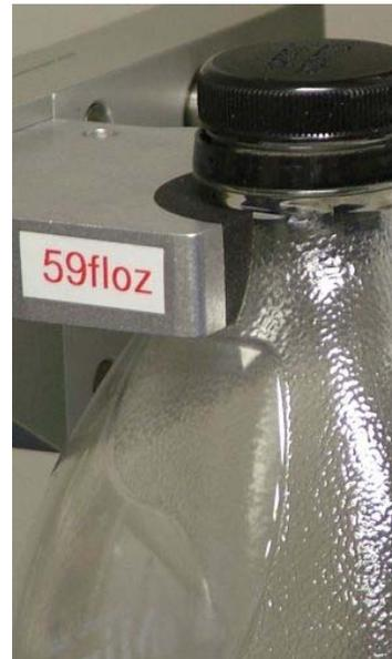
**Figure 18: Setup – Clamp height adjustment**
