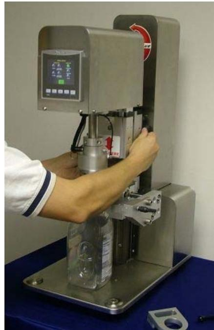
**Figure 20: Setup – Lowering the head**
