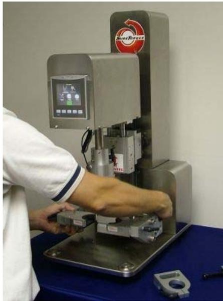
**Figure 15: Setup – Lowering clamps**
