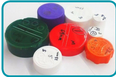
Varying cap sizes require multiple molded or serrated chucks
