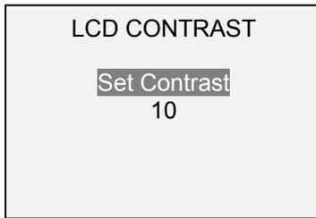
Press **ENTER** to modify the contrast. Select a value from 0 to 25, 25 producing the most contrast.
