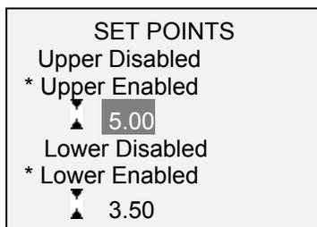
Either one, two, or none of the set points may be enabled. To toggle between clockwise and counter-clockwise directions, press the **DIRECTION** key.
